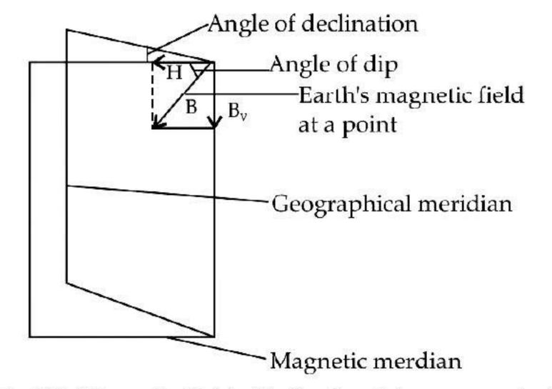
Horizontal Component of Earth's Magnetic field: The horizontal component of Earth's magnetic field H is in the horizontal direction in the magnetic meridian.
