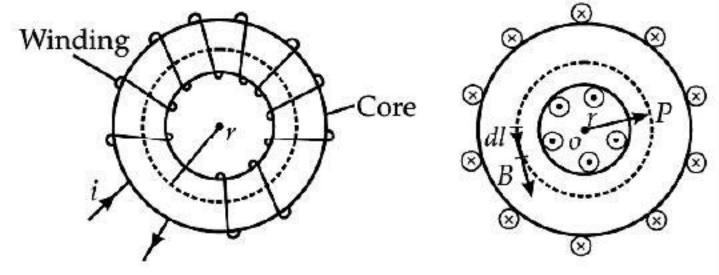
So, the magnetic field is only confined inside the body of a toroid in the form of concentric magnetic lines of force.
